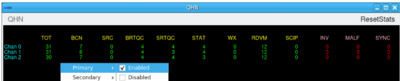
Figure 18. Dynamically Disable/Enable Radar Feeds
