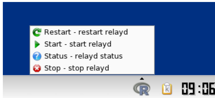
Figure 9. Manage relayd Through the Main Panel
